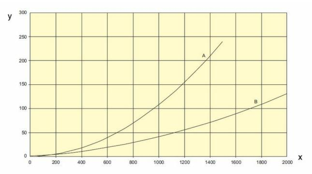
$Y = Pressure\ drop\ Pa/m\ X = Airflow\ m3/h\ A = \varnothing 150\ mm\ (8")\ straight\ B = \varnothing 200\ mm\ (8")\ straight$
